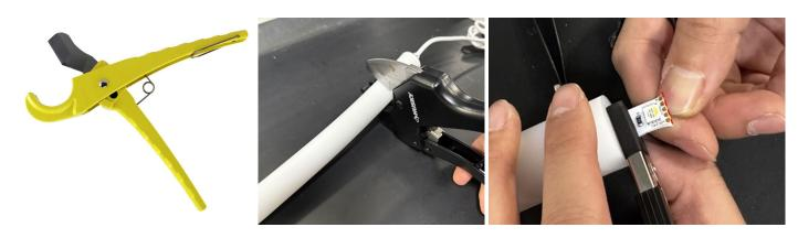
2. Fill the end cap (LN360-EC-W, LN360-EC-B) with silicone glue. Optional: Apply super glue to the perimeter of the end cap to speed up the bonding.
