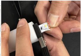
2. Use pliers to gently pull LED strips out of neon and clamp them in place.
